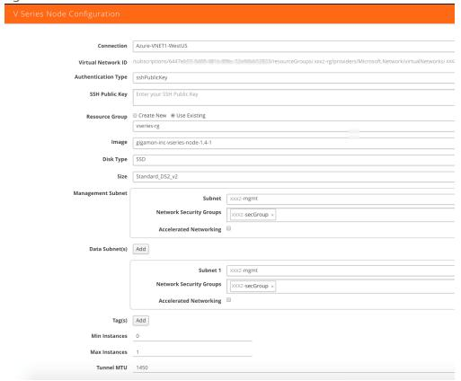
Figure 3: Configuring the GigaVUE V Series Node
